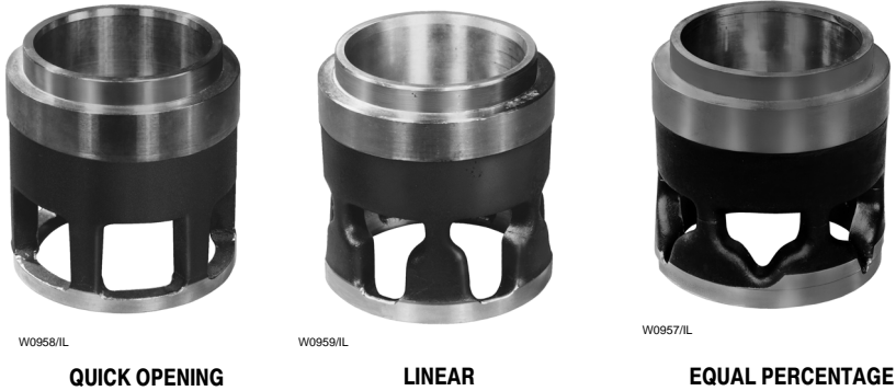
Figure 1-8. Characterized Cages for Globe-Style Valve Bodies
