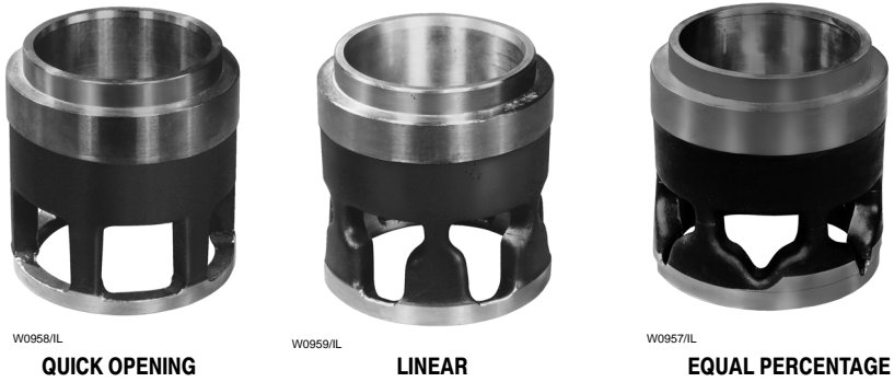
Figure 3-28. Characterized Cages for Globe-Style Valve Bodies
