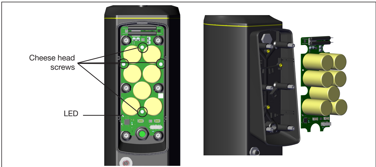
Image 14: Loosen screws on the printed circuit board/remove SAFEPOS energy-pack
