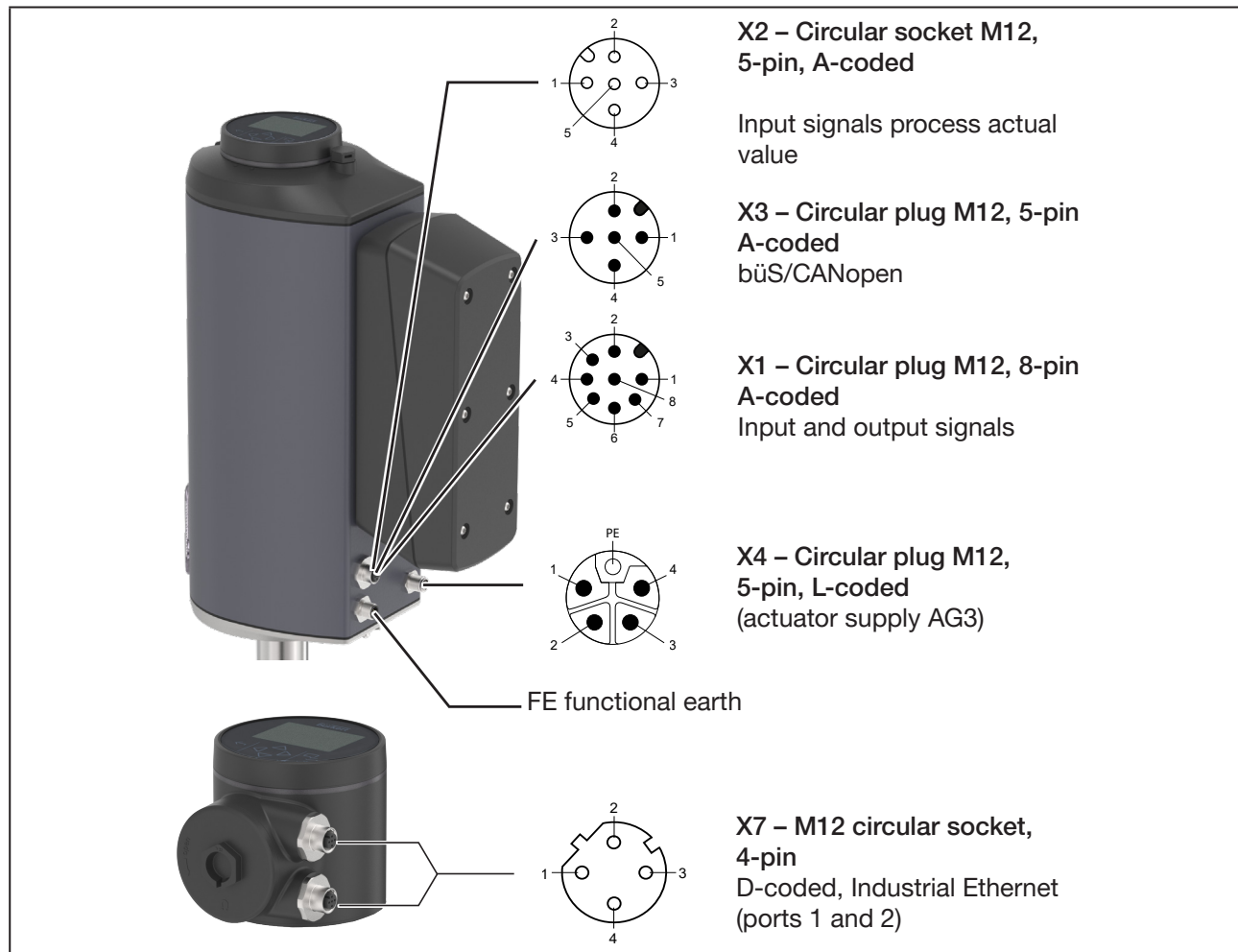
Image 28: Description of circular plug-in connector AG3
