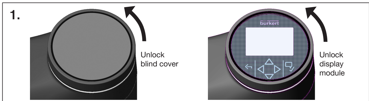
Image 31: Remove blind cover or display module
