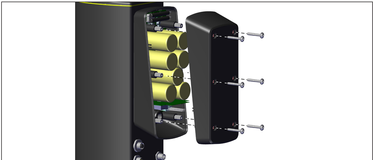
Image 12: Take off SAFEPOS energy pack cover
